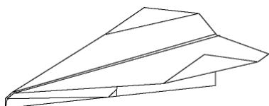
Fold the wings down along fold lines 6 and the winglets up along fold lines 7. Add wing dihedral by tilting the wings up slightly away from the fuselage. The wings will have a slight "V" shape when viewed from the front. Cut two slits, one inch apart, along the back edge of each wing to make elevator adjustments. Start out by trying some up-elevator. You are ready to fly!
