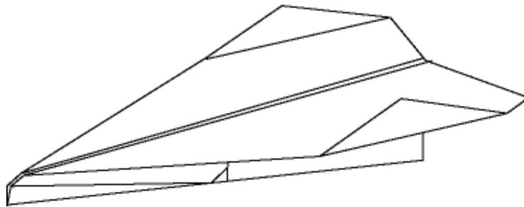
This plane is the classic schoolyard dart. It has short, compact wings and will fly straight as an arrow. It generally needs some up elevator along the back wing edges to fly properly.
