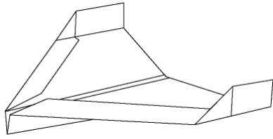
Fold the wings down along fold lines 5 and the winglets up along fold lines 6. Add wing dihedral by tilting the wings up slightly away from the fuselage. The wings will have a slight "V" shape when viewed from the front. Add elevator slits along the back edge of the wings to adjust the flight if necessary. You are ready to fly!
