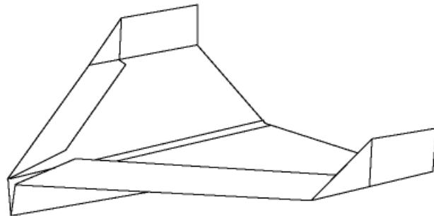
This plane produces tremendous lift at low speed, giving it a very low glide slope. It is an excellent indoor flier and will coast across the room on slow, smooth glides.
