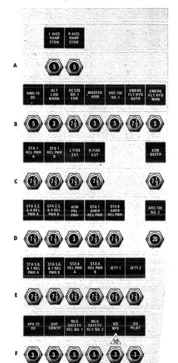
DC ESSENTIAL NO. 2 CIRCUIT BREAKER PANEL (RIGHT AFT) (PANEL NO. 7)
