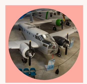
In addition to training pilots, crews aboard bombers also had to be trained in the air. The **AT-11 Kansan** was originally an airliner that was converted for use as a trainer for the Army Air Forces. The nose of the Beechcraft Model 18 was changed to clear Plexiglass and the fuselage was modified into a bomb bay capable of carrying 1000 lbs. of bombs. Bombardiers and navigators trained on Kansans throughout WWII up until the 1950s.
