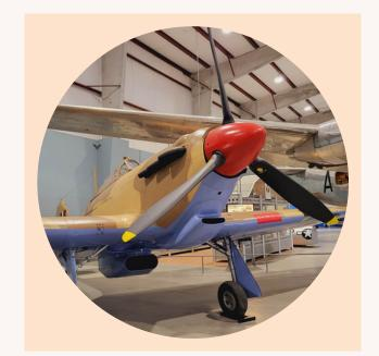
The Hawker Hurricane is a British fighter that first flew in 1935. It was the first British fighter that was a monoplane (one wing on either side) and the first to feature retractable landing gear. It had much heavier firepower than other British fighters, with eight machine guns mounted on the wing. The Hawker Hurricane bore the brunt of the fighting during the Battle of Britain, when the German Air Force (Luftwaffe) attempted, but ultimately failed, to gain air superiority over Great Britain.
