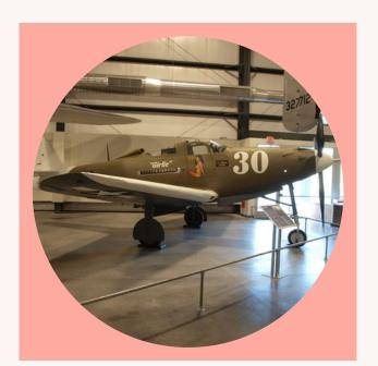
The P-39 Airacobra has several unique design features, including an engine behind the pilot, automobile-type doors, and tricycle landing gear. The P-39 had great performance at low altitudes, but was ill-suited to flying at high altitudes. The large 37 mm cannon mounted on the nose made them excellent ground attack aircraft however, and the US sent large numbers of P-39s to the Soviet Union under the Lend-Lease Act for this purpose.
