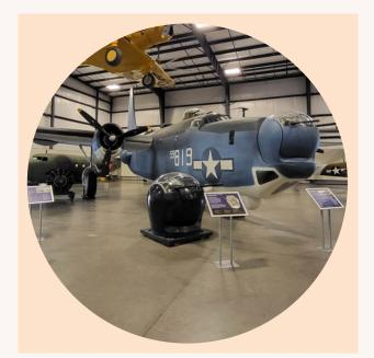
The PB4Y-2 Privateer is a long-range patrol bomber based on the B-24 Liberator. Some differences include a single tail, more armament, a stretched fuselage, and state of the art radar and navigation equipment giving them all-weather capability. They flew anti-submarine and anti-shipping missions in the Atlantic and the Pacific. After WWII, they also served as weather reconnaissance and signal intelligence gathering. Some served as aerial tankers fighting forest fires through 2002.
