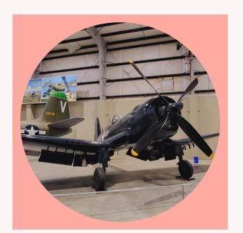
The F4U Corsair has one of the most recognizable designs of any fighter aircraft ever. The Corsair was a carrier-based fighter used by the United States Navy. The massive engine and corresponding large propeller required the distinctive inverted gull wing to give enough clearance for the propeller to spin. Corsairs had the longest production run of any American aircraft from WWII, with the last one being built in 1952. The US Marines used later versions of the Corsair during the Korean War.
