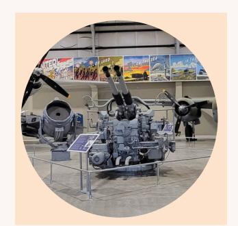
The Twin Bofors 40mm was one of the most widely used anti-aircraft weapons of WWII. Originally designed in Sweden, the US Navy acquired a license to build them with modifications including, converting the targeting units from metric to imperial, updating ammunition, powered mounts, and adding a liquid cooling system. By the end of WWII, Bofors 40 mms were found on almost every American ship. Some were used by the US Air Force aboard their AC-130 gun ships as late as 2019.
