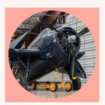
The TBM Avenger was the main torpedo bomber used by the US Navy during WWII. Originally designated TBF, the company that designed them, Grumman, could not keep up with the Navy's demand for Avengers. As a result, they asked General Motors Company to convert one of their assembly lines used for making vehicles to make Avengers. Like many carrier-based aircraft of the time, the Avenger's wings fold backward to give more space to store the planes on the carriers.
