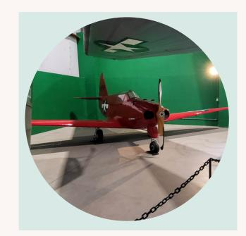
Behind the Skytrain is a small red plane, the **PQ-14 drone.** These all-wooden drones could be flown remotely or by a pilot. The remote feature meant that these were useful for target practice for anti-aircraft gunners in the US Navy and Army.
