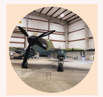
The IL-2 Shturmovik was a Soviet plane used for ground attack. Faced with a severe shortage of aluminum, the plane was built with its wings and tail section made from wood. The nose and cockpit were heavily armored, making them difficult to shoot down from the ground. They were vulnerable from the air however, and thousands were lost during the war. While not technologically advanced, the IL-2 became the most produced aircraft of WWII, with an estimated 36,000 of them built.
