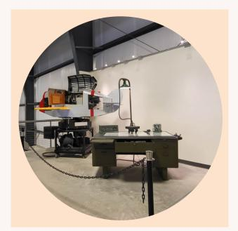
At the top of the stairs on the mezzanine, you will find a **Link Instrument Trainer.** A series of bellows, pumps, and valves allowed the trainer to simulate aircraft movement. Using the trainer was safer and cheaper, because the student wasn't using an actual aircraft that required fuel and maintenance. The Army Air Corps began using them in 1934 and implemented a hood, so the pilot would have to use the instruments in the "cockpit" to fly, and not rely on visuals while flying.
